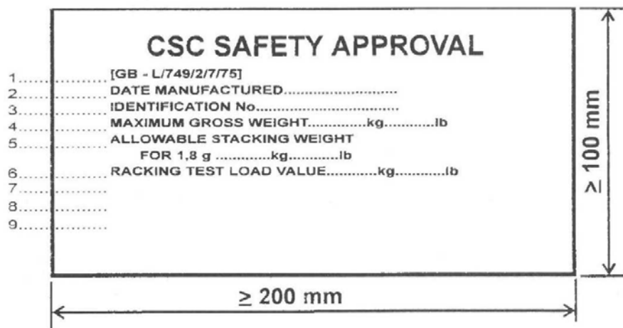
Figure 8.10.7-4: Safety approval plate on container
