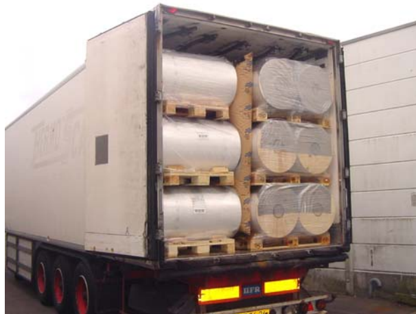
Picture 18: Filler between the rows of cargo
