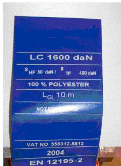
Picture 38: Label in accordance with standard EN12195-2
