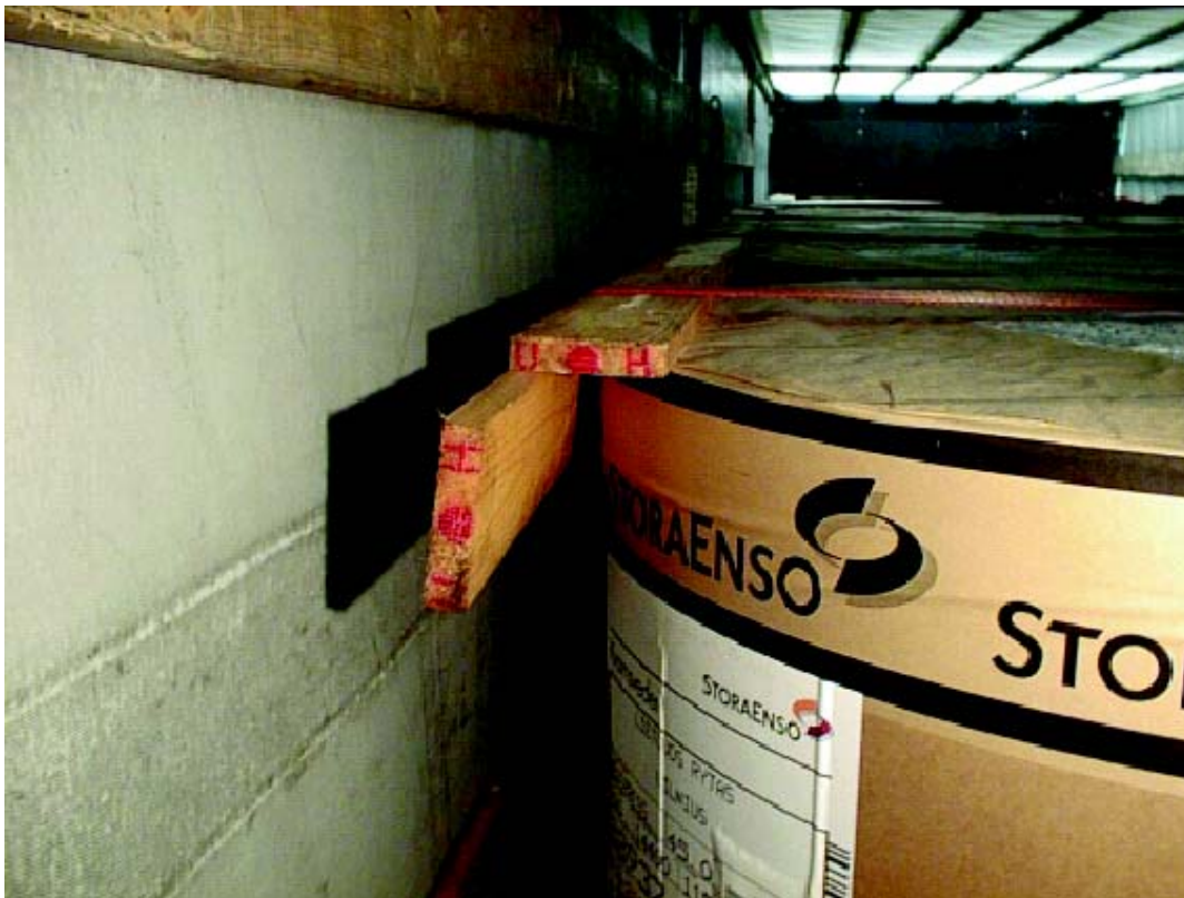
Picture 53: Edge beam made of wooden boards.
