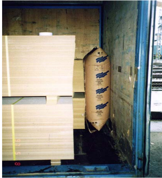
Picture 19: Air cushion in a semi trailer
