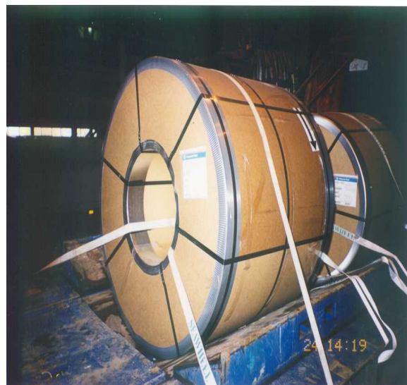
Straps through and across the coil
