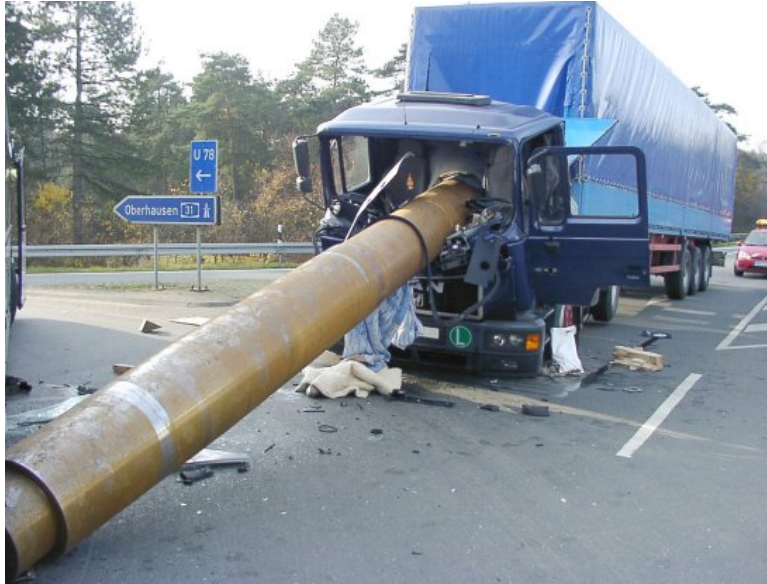
Picture 1: During heavy braking, the badly secured steel tubes made their way through the headboard and the drivers cab.
