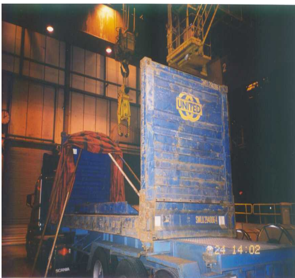
Flatrack with a cover and groove
