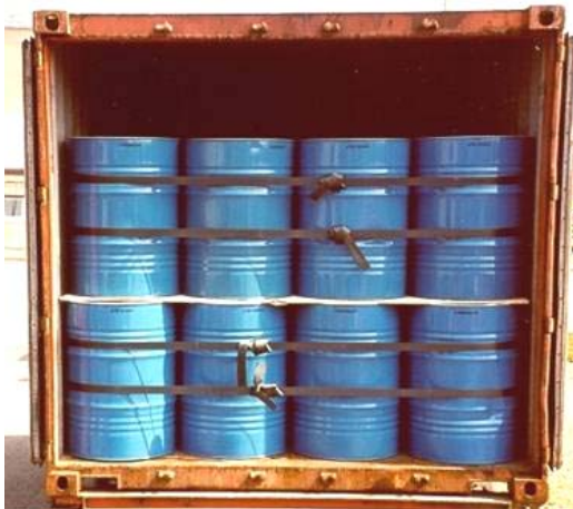
Picture 89: Loose drums double-stacked in a container, two layers of four rows
