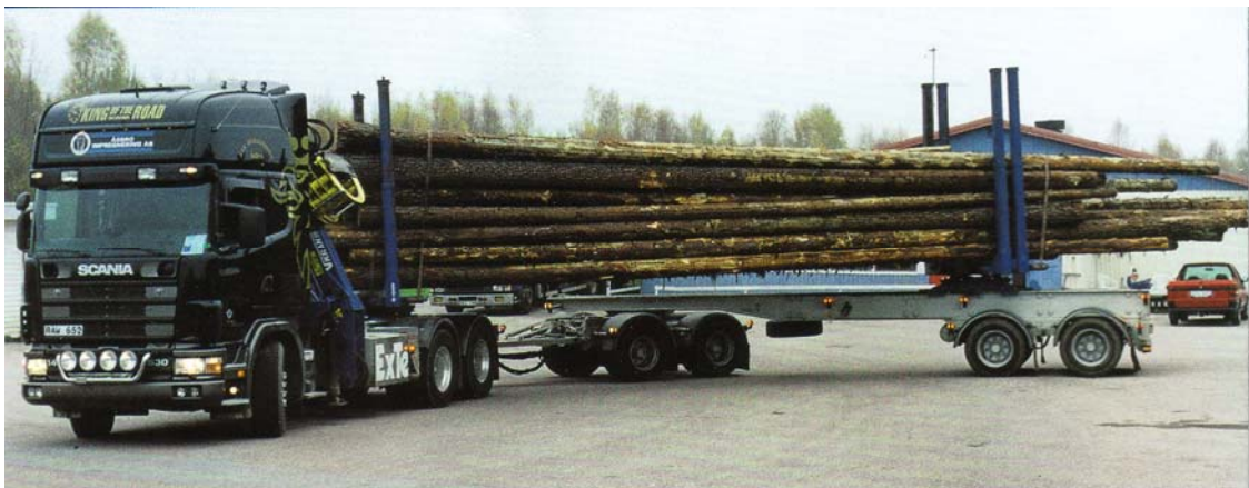
Picture 82: Transport of whole trees (This is a special purpose vehicle not complying with Directive 96/53/EC)
