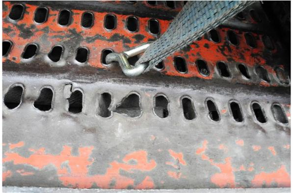
Regularly inspect the check plate for wear and tear.
